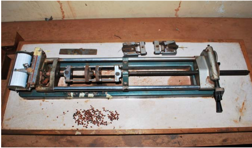
Figure 3. Universal Testing Machine (Monsanto Tensometer) with Prosopis Africana Seed under test.
