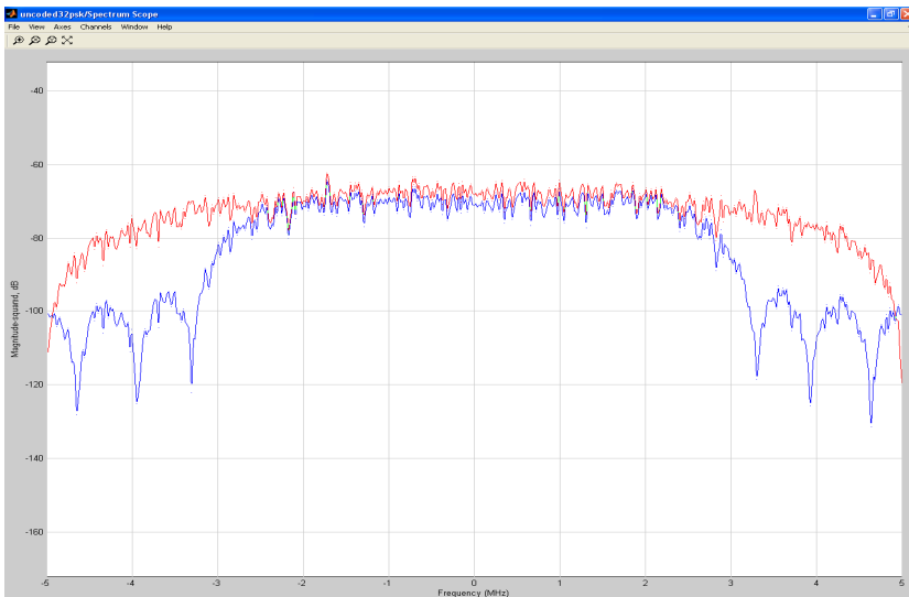
Figure 4.13 Spectrum Scope of Convolution Coded 32-PSK at 5.5 MHz
